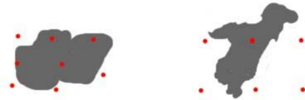
Figure 1. Control points (red) evenly distributed. To the left, they surround – or cover – the most of the features that are of interest to analyze/digitize (here symbolized by grey area). To the right, those features are outside of the control points, and there is a greater risk that the transformation includes more errors on these features.
